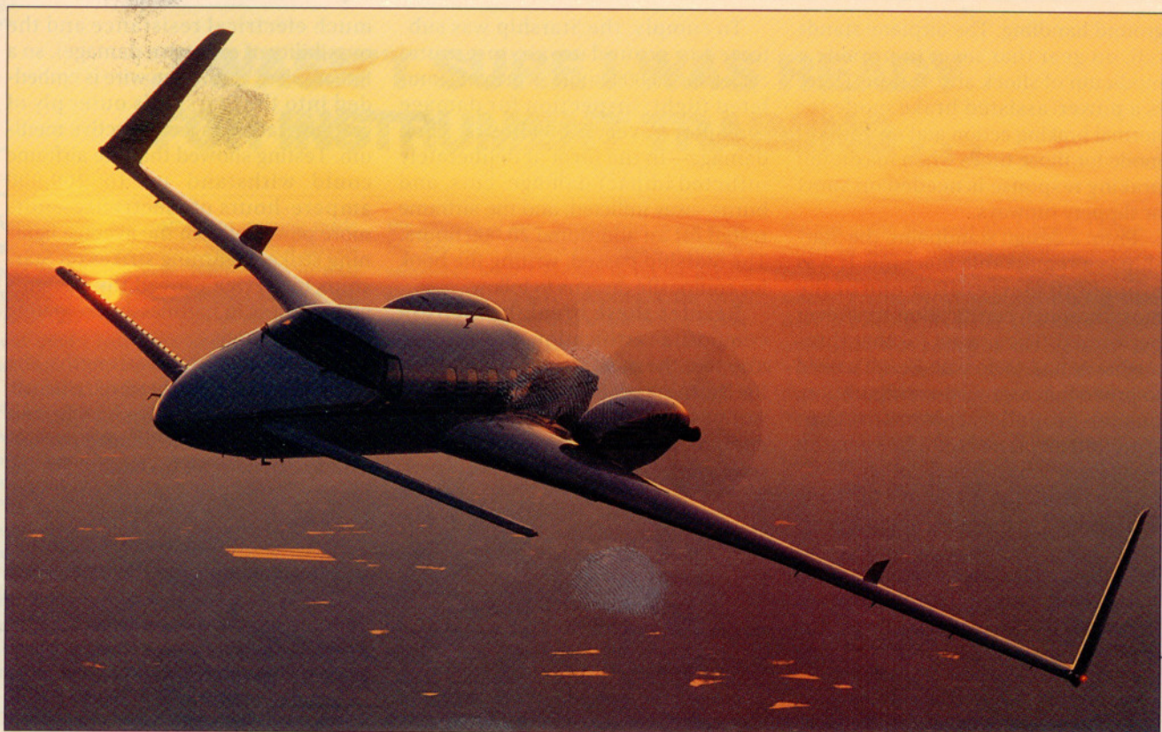
Ramp-watchers can spot a 2000A by its big exhaust stacks and lack of canard stall strips.
